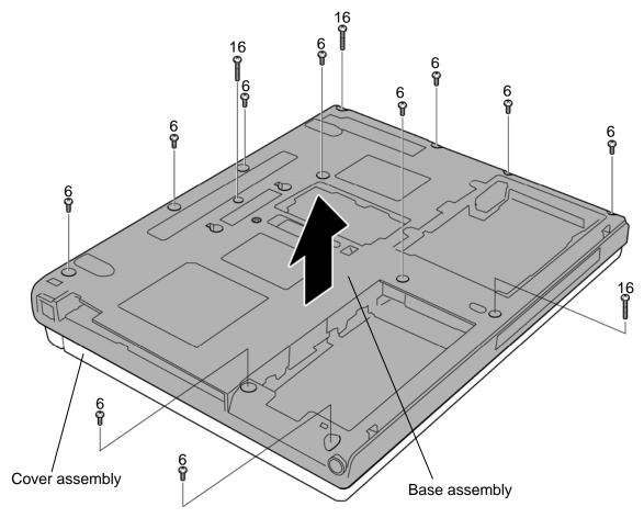
Figure 4-26 Removing the base assembly and cover assembly (3)
